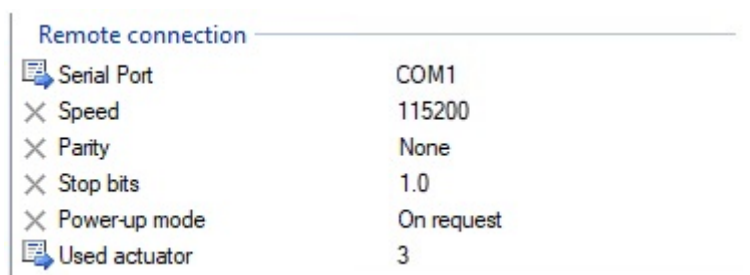
Fig. 14 – Remote port configuration example (modem).
